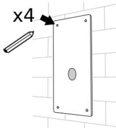
Drill the four fixing holes with a 6 mm drill bit and insert the wall anchors:
