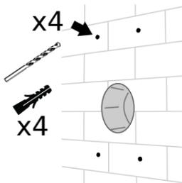
Using a screwdriver, pierce the rubber cap and feed the wires through:
